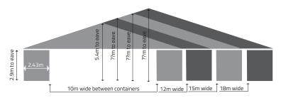
10m portal width with 5m portal bay increment | eave 2.9m 12m portal width with 5m portal bay increment | eave 2.9m 15m portal width with 5m portal bay increment | eave 2.9m 18m portal width with 5m portal bay increment | eave 2.9m
