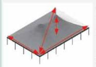
For best fit ensure the tent is properly erected. Ensure eave line is tensioned to design dimensions. Ensure that the tent is square. Ensure the centre poles are set to design height and in their correct vertical position.
