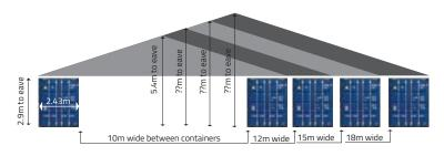
10m portal width with 5m portal bay increment | eave 2.9m 12m portal width with 5m portal bay increment | eave 2.9m 15m portal width with 5m portal bay increment | eave 2.9m 18m portal width with 5m portal bay increment | eave 2.9m
