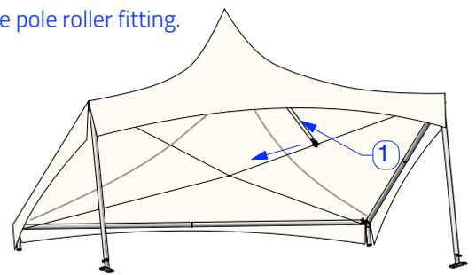
7. - Raise onto legs with erecting fork at centre of eave.
