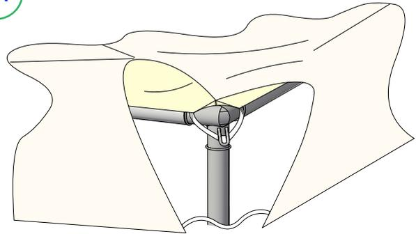
5. - Button lock base fitting to leg alloy.
