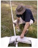
Attach the Push Pole and check that the Retaining Clip and Cord are secure.
